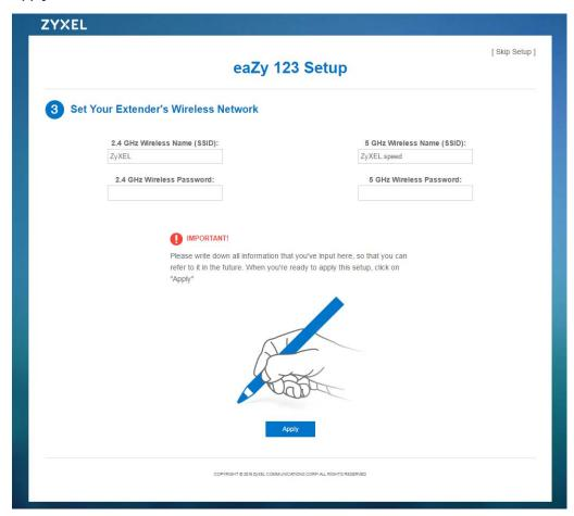
The eaZy 123 setup wizard is complete. Verify the WRE6505 v2's wireless network settings and click **GO** to log into the web configurator again.
