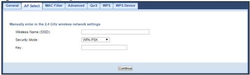
Configure the wireless settings between the WRE6505 v2 and its wireless clients. The WRE6505 v2 automatically copies the SSID of the associated AP and appends ".speed" to the 5GHz SSID. Click Apply to save settings and restart the WRE6505 v2.
