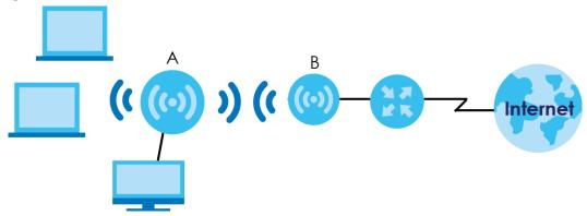
After the WRE6505 v2 and the access point connect, the WRE6505 v2 acquires its IP address from the access point. The clients of the WRE6505 v2 can now surf the Internet.
